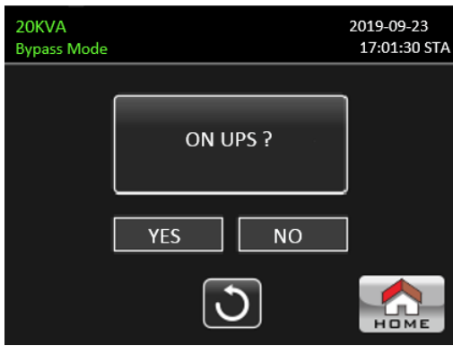
TURN ON UPS
